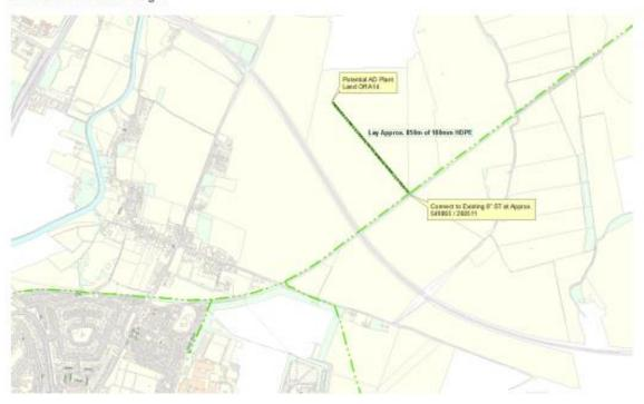
The connecting pipeline of 850m of 180mm High Density Polyethylene has been designed to maintain an acceptable velocity and an acceptable pressure drop (<10mb) for an Entry Connection with a source pressure (Bio-methane injection point) of between 3.5 – 7barg.
